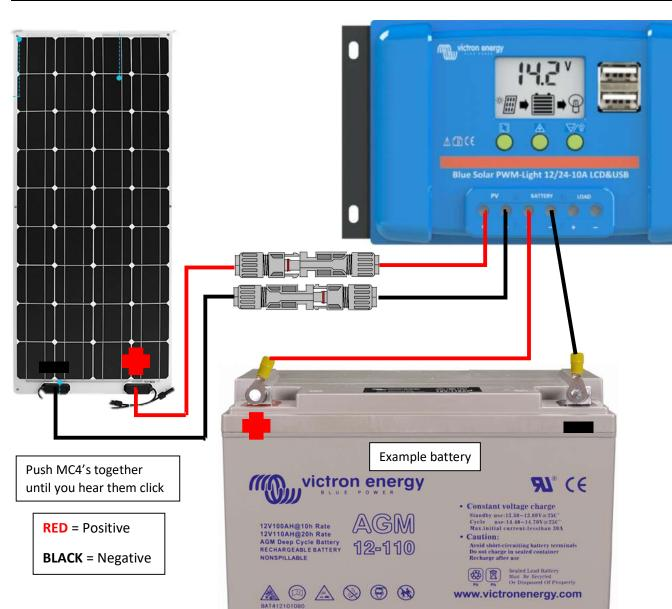
Connect the battery cables first, then the solar.
